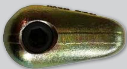
**[EN]** Fixed joint suitable for joining both steel pulling ropes and synthetic pilot ropes, made of galvanized high tensile steel, with a design fit for easy and safe passage through the bullwheels grooves of winches, screwed pin closing device provided of concave spacer to facilitate the loop of rope position.
